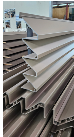
Factory extruded and folded aluminium plank.
