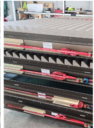
Aluminium planking unitised panels with end caps, stacked on factory crates ready for transport.
