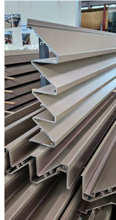
Factory extruded and folded aluminium plank.
