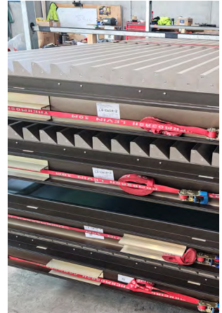
Aluminium planking unitised panels with end caps, stacked on factory crates ready for transport.
